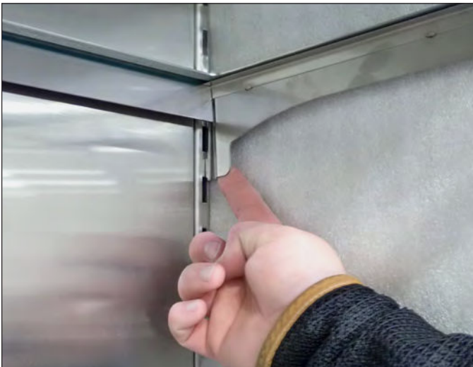
FIG. 6. Push the bottom tab inward.
