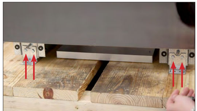
FIG. 7. Shipping bracket bolt locations.
