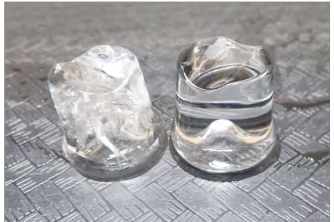
FIG. 1. Recently produced ice cubes may have cracks through the ice (see left cube). This is normal ice production.
