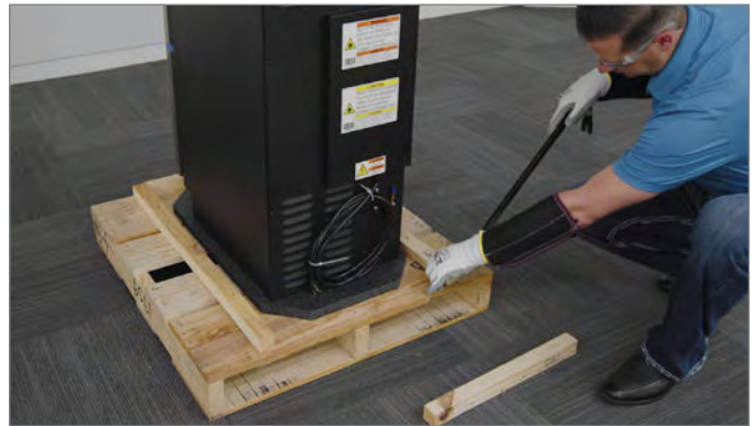
FIG. 2. Pry the runner boards off the skid.
