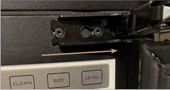
FIG. 1. Slide the door off the hinge bolts through the keyhole slots.
