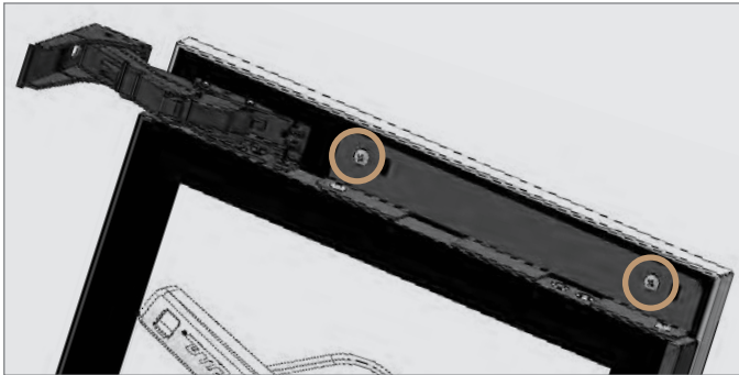
FIG. 1. Spacer / top door bracket screw locations.
