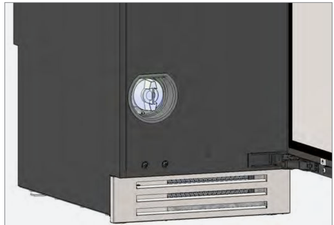
FIG. 3. Installed water filter.
