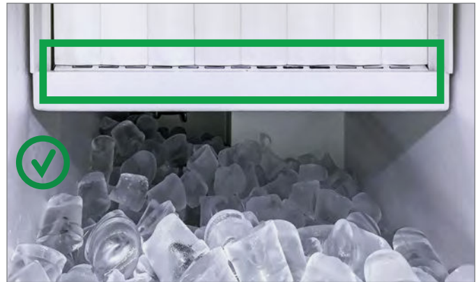
CORRECT. Ice guide finger holes are hidden; ice guide slotted holes are visible.
