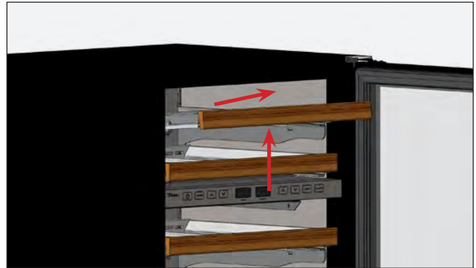
FIG. 1. Lift and pull the wine rack forward.
