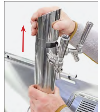
FIG. 5. Lift the top off the draft standard.
