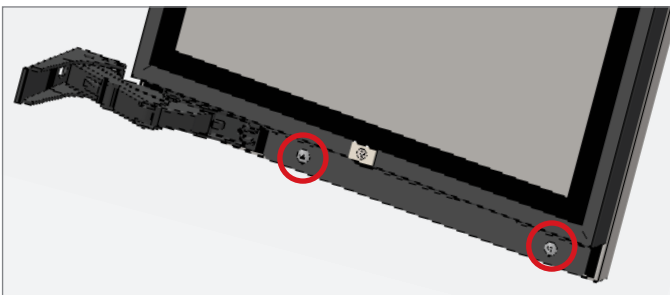
FIG. 2. Bottom door bracket screw locations.
