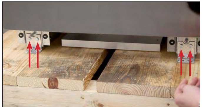
FIG. 7. Shipping bracket bolt locations.
