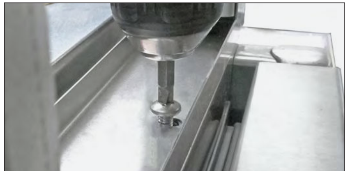
FIG. 10. Remove the screws from the metal channel.
